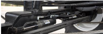
Sprayflex High Rise Axle with Hydraulic Steering
