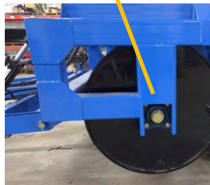
3" Shaft and Bearings
